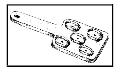
In some fish processing operations such as salting and smoking it is convenient to remove the fish scales. A fish scaler made from bottle tops is easy to use and works even better than the back of a knife.
