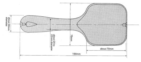
2. Four holes are drilled in the square head in a 3 cm square. These holes are enlarged using a 7/8" or 22 mm diameter bit.
