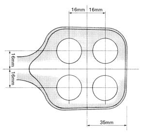
3. The wood between these holes is then cut away with a chisel to make a square in the middle of the block as in the diagram.
