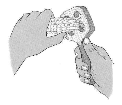
1. A piece of knot free hardwood about 19 cm X 7½ cm and about 3 cm thick, is shaped so that it has a rounded square head and a handle that is comfortable to hold, as in the diagram.
